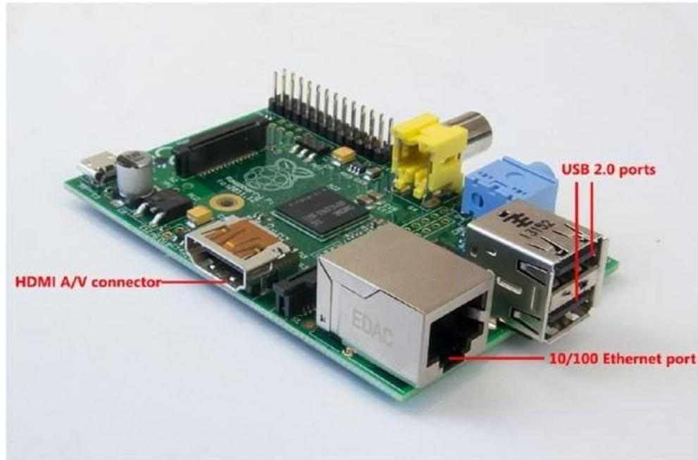
**Gambar 1-5** Port HDMI Raspberry Pi Model B, port Ethernet, dan port USB 2.0 ganda
