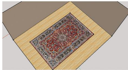
Figure 7-44: A rug photo was imported as an image, exploded, and turned into a component. It was then moved to the floor, where it flashed (top graphic). The editing box was opened, and the rug push/pulled up a bit to stop the flashing.
