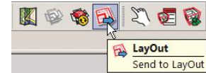
Figure 9–23: Click the Export to LayOut tool to send the model to LayOut.
