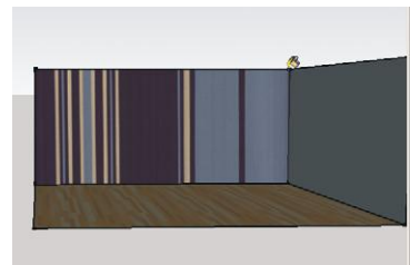
Figure 7–30: Click the texture on a face. Textures can only be applied to faces, not to blank space.
