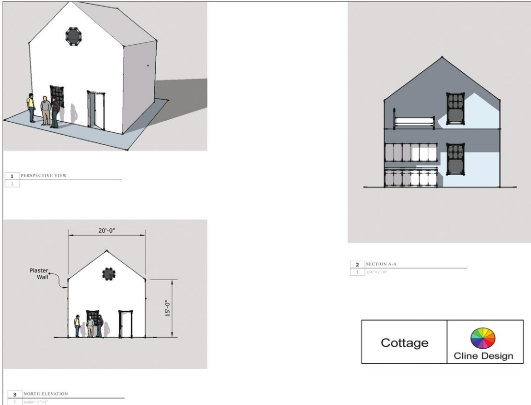
Figure 9–18: LayOut, a construction documents program, can display multiple views of a model simultaneously.
