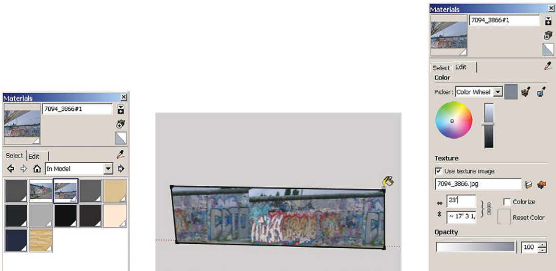
Figure 7-58: Paint the new texture onto a face and then edit its scale.
