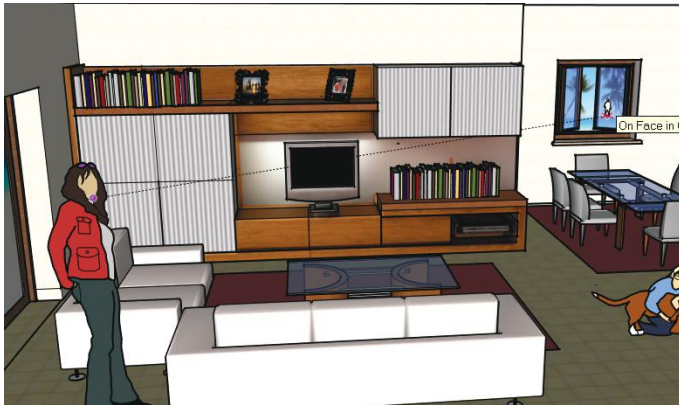
Figure 8–46: Click Position Camera on the scale figure's face, and drag the mouse to whatever you want her to look at. Then release. The model will shift to that view.
