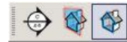
Figure 5-55: The Section toolbar. Its icons toggle the plane and cut displays on and off.
