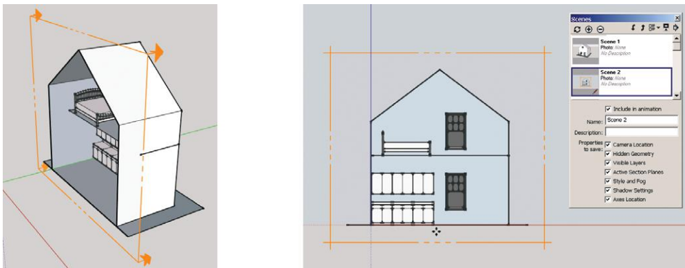
Figure 9–20: Make orthographic sections with the Section tool and the camera parallel projection setting.
