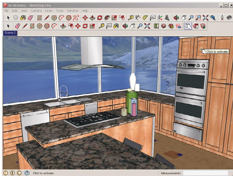
Figure 1-7: Clicking on this dynamic cabinet component makes the door open to show storage options.
