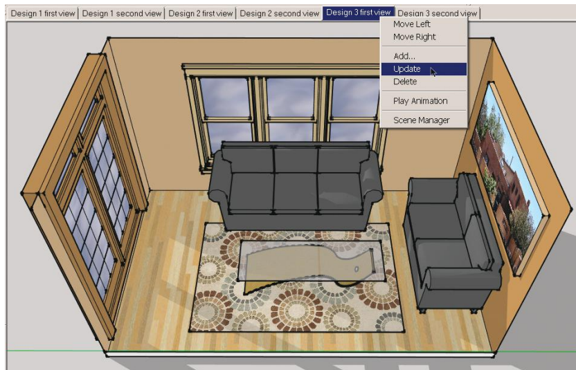
Figure 8–38: Make a fifth scene tab, create the scene, and then update the tab.
